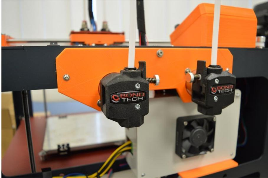
I am a big friend of the “BondTech” Extruder (<http://www.bondtech.se/en/start/>). These extruders offer most grip and extrusion force, great for “difficult” materials.
